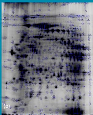
Automatically detected spot pattern of the Gel.
