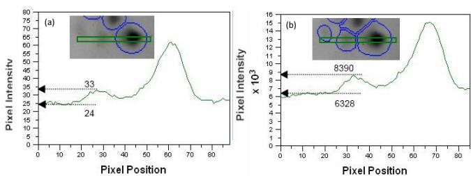
Figure 1. (a) Spot detection has missed spots due to the low difference in intensity between the spot and background noise. In the use of 16 bit images (b) the spots have been identified as there is a significant difference in intensity. An increase from 9 to 2062 levels above background intensity.
