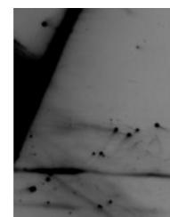
Figure 3. Top left corner of blot image, identification of spots is difficult to distinguish due to the presence of non-spot features, noise and streaking.
