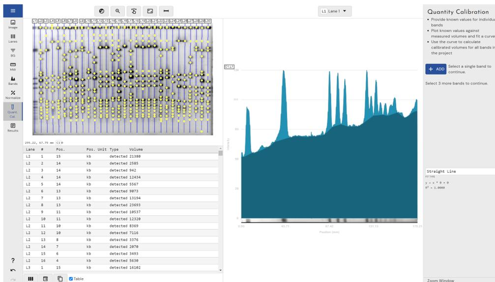
The quantity calibration mode is used to convert detected band volumes to real-world values by including known value standards in your gel/blot experiment and then defining those values within Phoretix 1D.
