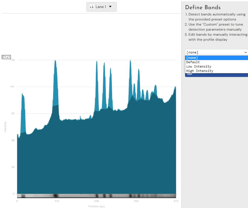
"Low Intensity" is designed to detect fainter bands for analysis
