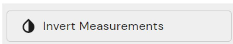
The invert measurements button below the channel names inverts the measurements for all channels in the image. Use if all channels are displaying bands (or signal) as troughs instead of peaks.
