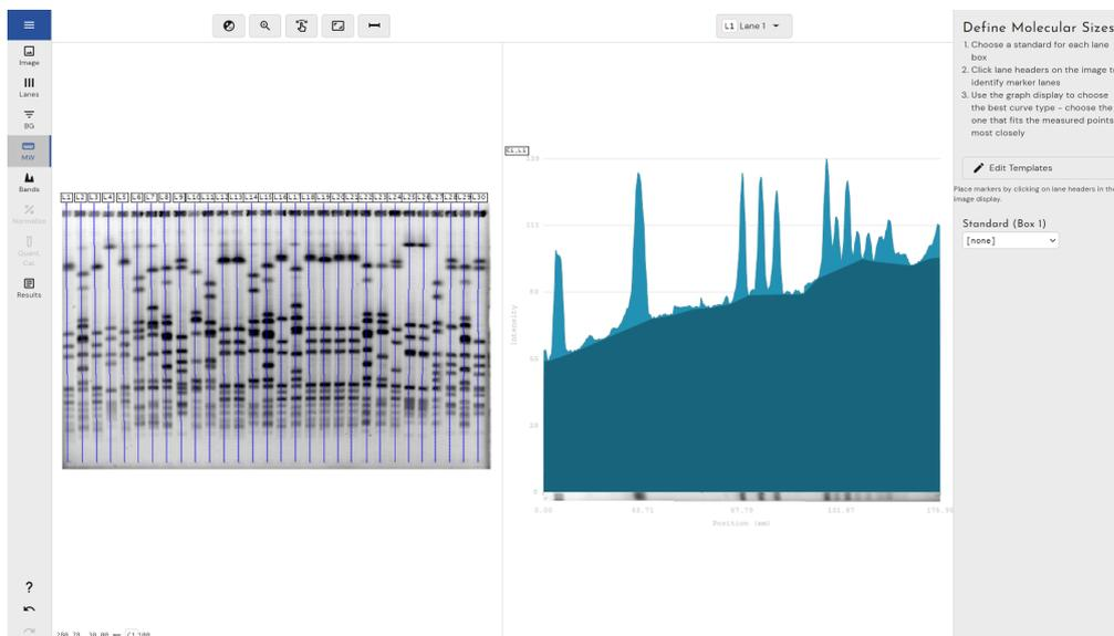
The Molecular Weight Calibration Window uses a standard lane within your lane box to determine the molecular weight of all the bands across the whole lane box.
