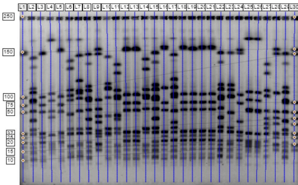
As you can see, when multiple MW standards are present on an image they attempt to join across the image. These are used as reference points for MW calculation and any distortions in the gel can be accounted for mathematically by taking into account how the standards have moved at either end.
