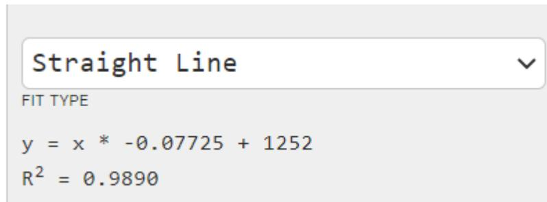
*Whilst at least 3 bands with known values are required to create a calibration curve, Phoretix 1D supports a virtually unlimited number of known band values to create your calibration curve. The greater the number of standards that form the calibration curve the greater the accuracy of that curve and therefore the greater the accuracy of the interpreted (unknown) band values derived from it.*
