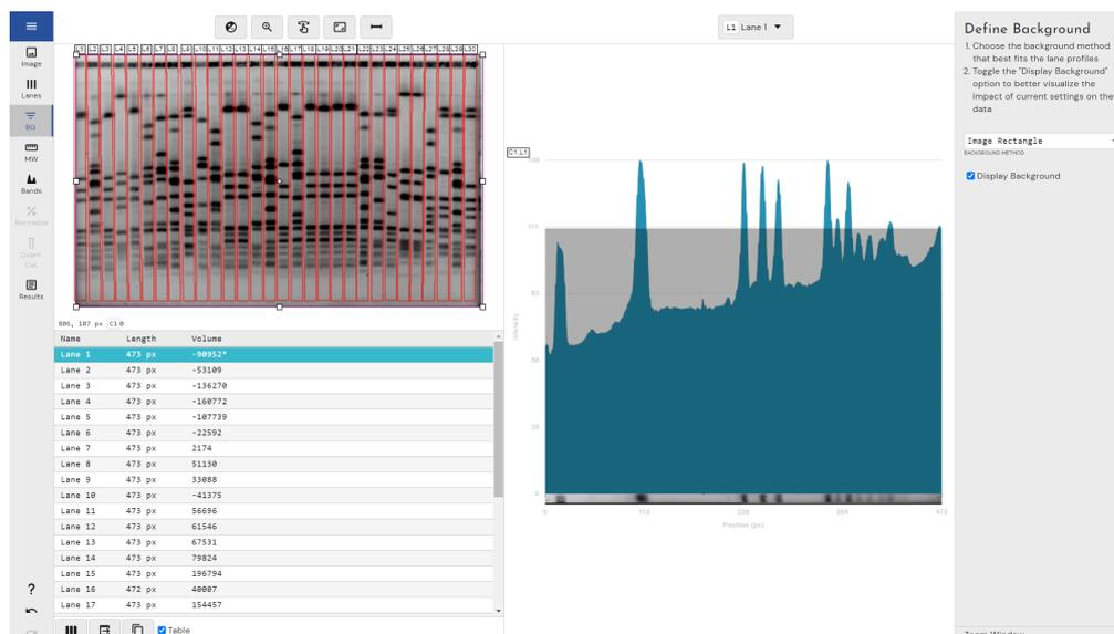
Use the handles on the edges of the rectangle to resize it and the diamond handle in the center to move it. From this rectangle, the background intensity is applied and calculated for all lanes.
