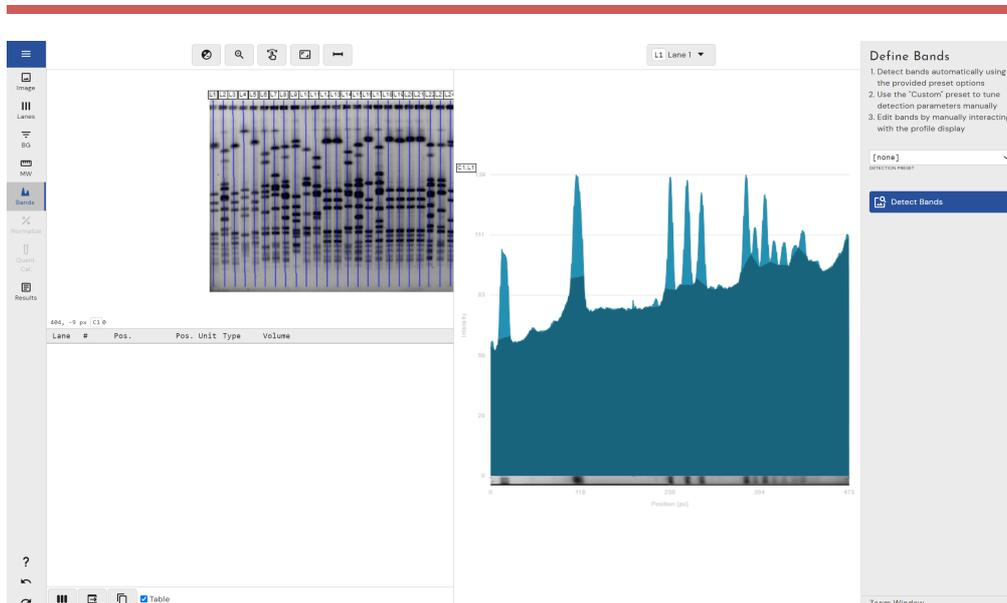
The Bands mode offers you automatic methods for detecting bands and also allows you to edit those bands manually after detection.
