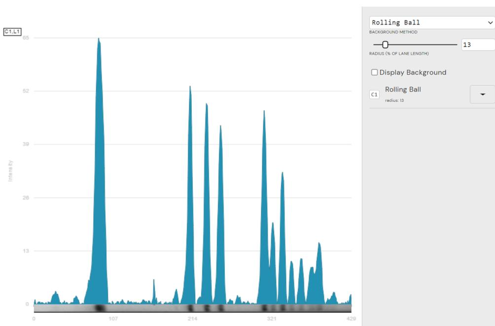
Display background checkbox unticked, lane profile is shown with background subtracted based on current background subtraction settings.
