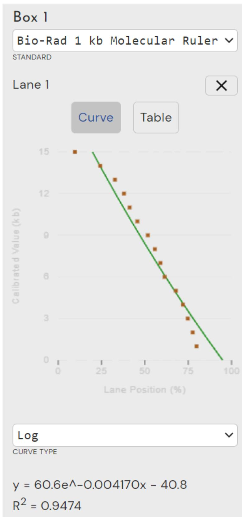
Where the orange diamonds are your known MW values (i.e. the steps in your MW marker) and the green line is the calculated values according to the selected equation.
