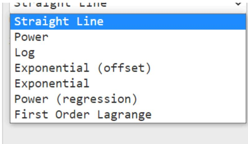
From the drop-down list, select the curve fitting type that most accurately reflects your data points (as a rule of thumb, this is usually the curve type that has the highest R2 value, the closer to 1 the better).
