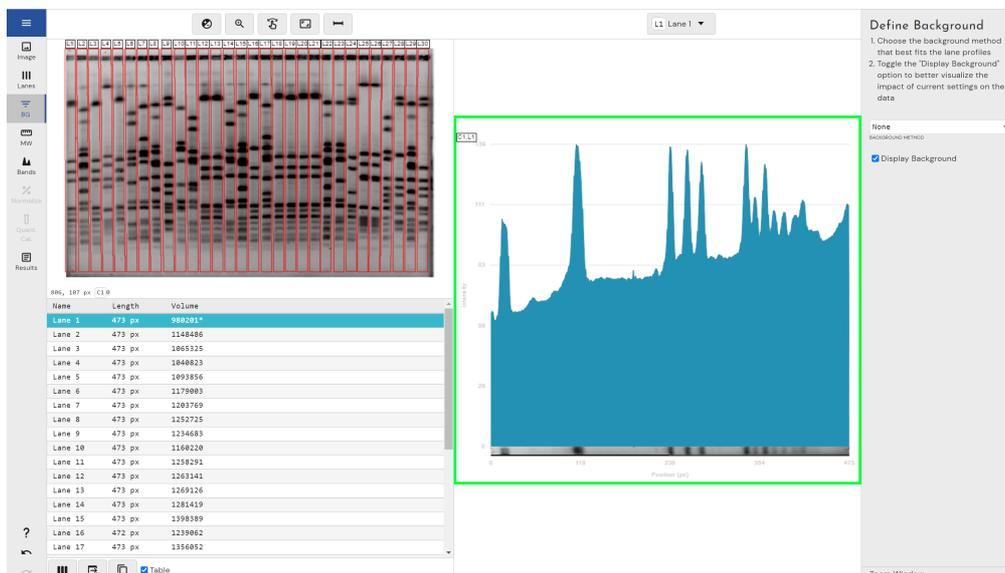
This mode allows the user to define the sensitivity and algorithms used for background subtraction.
